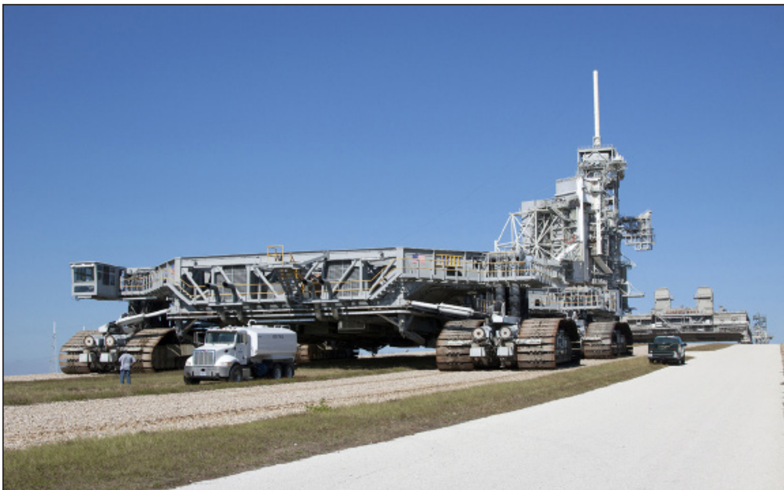
Crawler-transporter 1 approaches the top of Launch Pad 39A after traveling along the crawlerway at Kennedy Space Center on Dec. 3. New jacking, equalizing and leveling, or JEL, hydraulic cylinders were installed on CT-1 and are undergoing a leveling and turning test as the crawler travels along the slope. Photo credit: NASA/Daniel Casper
