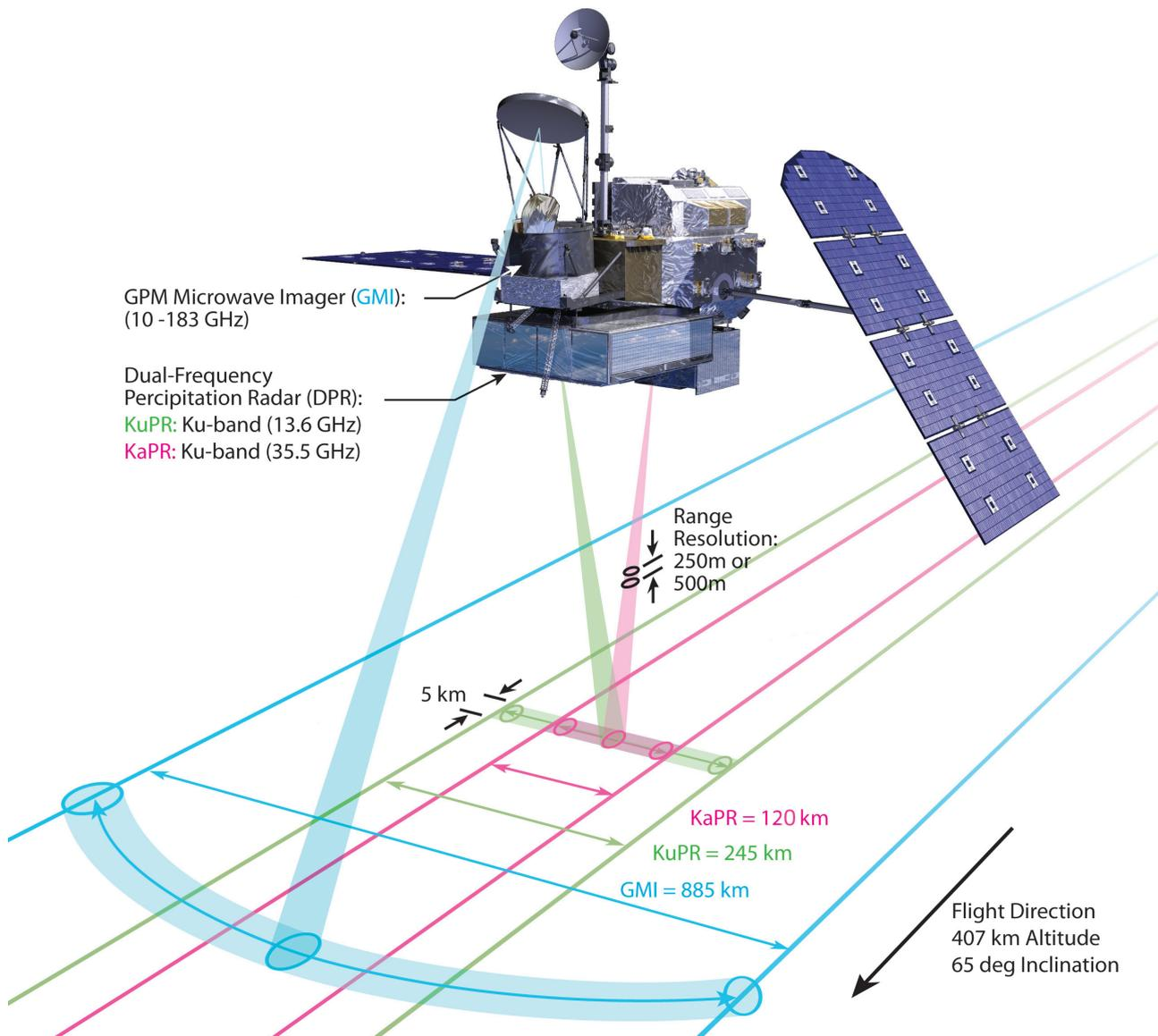
Diagram of swath coverage by GPM sensors
