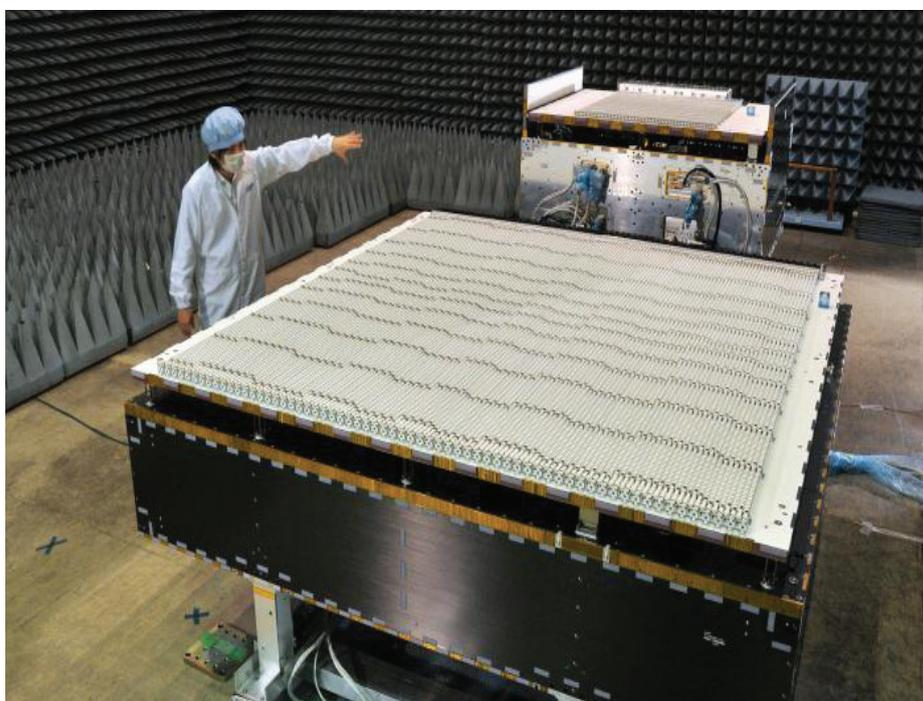
*A JAXA scientist standing next to the Dual-frequency Precipitation Radar (DPR) instrument. The Ku-band radar is in the foreground and the Ka-band radar is the smaller one in the background.”*
