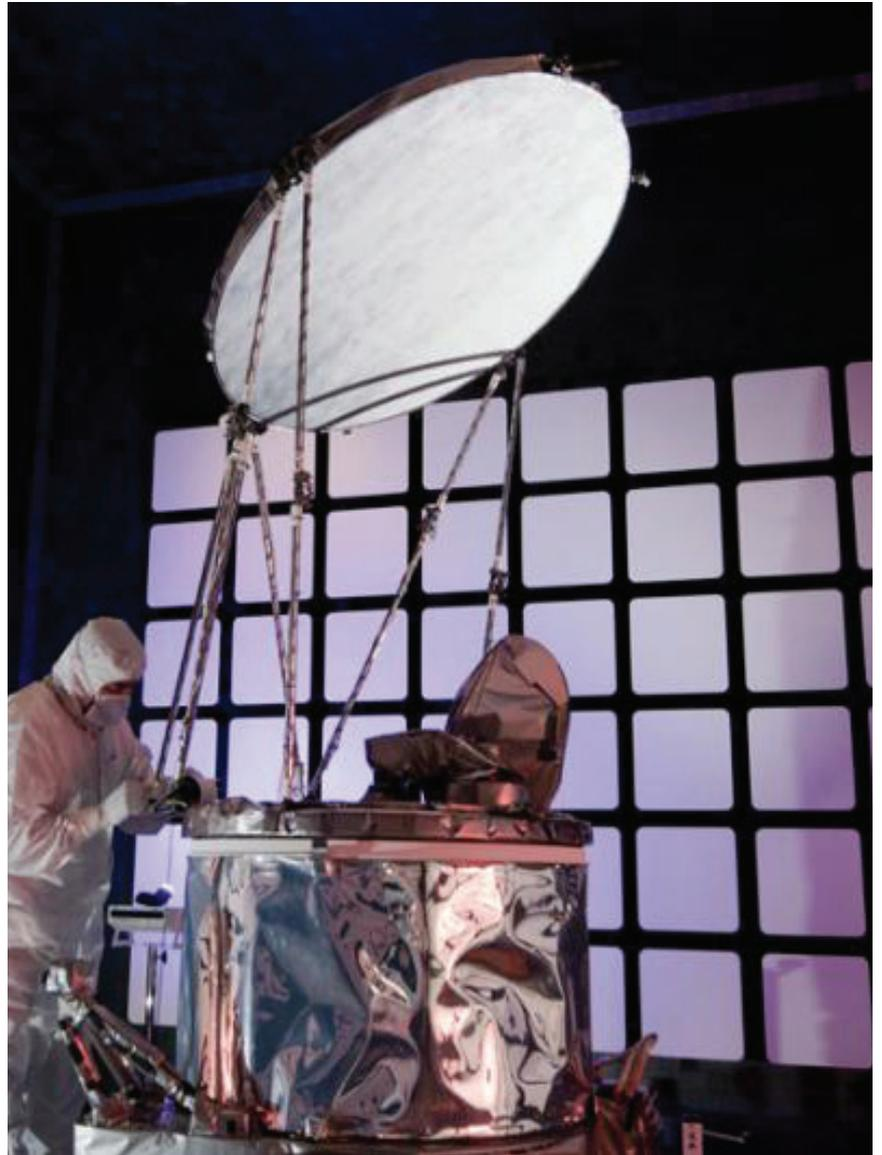
*GMI undergoes electromagnetic interference and compatibility testing at Ball Aerospace & Technologies Corp.*
