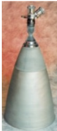
HiPAT Aerojet Rocketdyne MON-3 / MMH
