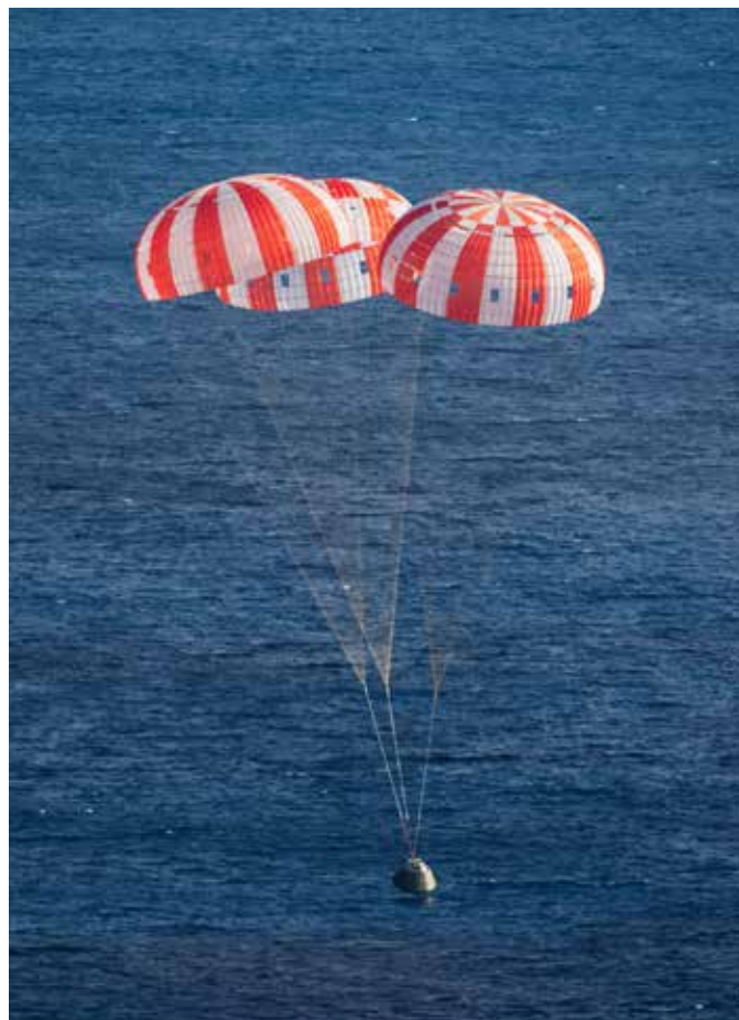
NASA's Orion spacecraft is lowered gently to the Pacific Ocean under its three massive main parachutes at 11:29 am EST on Dec. 5, 2014. Orion launched on its first test flight at 7:05 am and over the course of two orbits and 4.5 hours, traveled 3,600 miles above Earth to test systems critical to human deep-space exploration.
