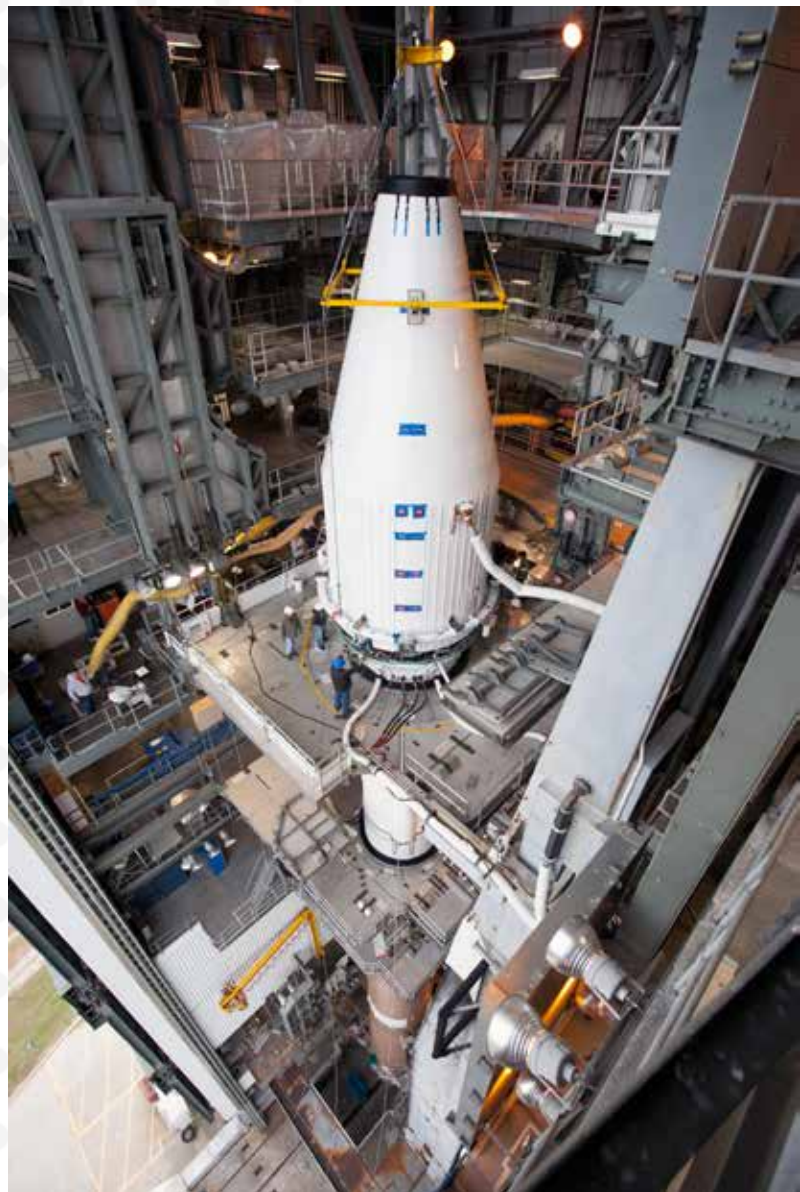
Crews guide NASA's MAVEN spacecraft, inside a payload fairing, into place atop a United Launch Alliance Atlas V rocket at the Vertical Integration Facility at Space Launch Complex 41. The Atlas V will lift MAVEN into space and on to Mars. MAVEN is short for Mars Atmosphere and Volatile Evolution.
