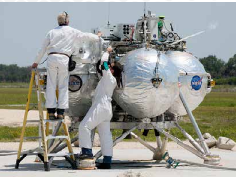
Technicians check out NASA's Project Morpheus prototype lander, which just touched down on a dedicated pad inside the ALHAT hazard field near the Shuttle Landing Facility at Kennedy Space Center in Florida. The efforts in Advanced Exploration Systems pioneer new approaches for rapidly developing prototype systems, demonstrating key capabilities and validating operational concepts for future human missions beyond Earth orbit.
