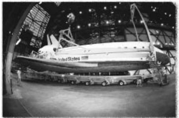
The orbiter Columbia, shown in preparation for mating to its solid rocket boosters and external tank, flew twice during FY 98.
