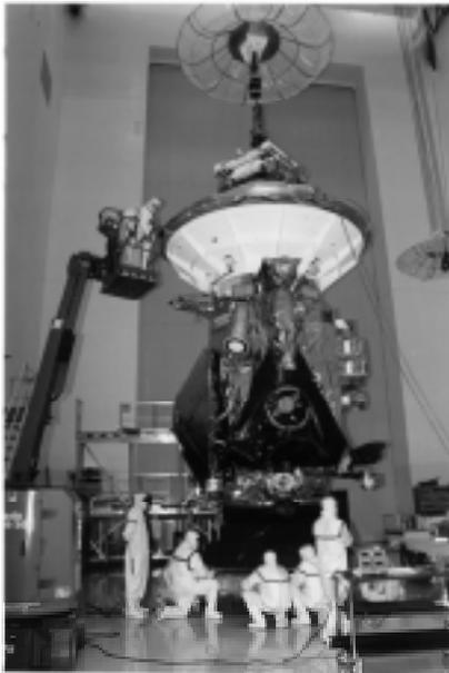
*The Saturn-bound Cassini spacecraft is lifted inside a KSC processing facility in preparation for its transport to the launch pad at adjacent Cape Canaveral Air Station.*
