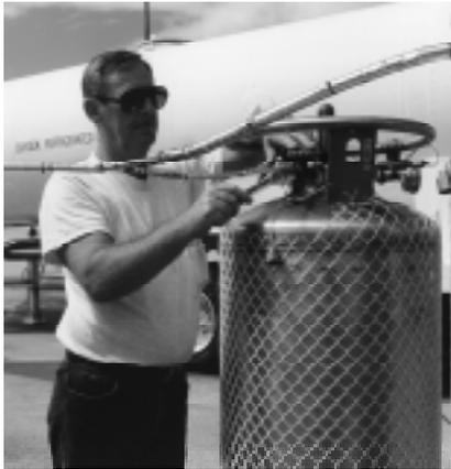
*A KSC technician connects a liquid air mixing device to dewars of liquid nitrogen and liquid oxygen. The mobile liquid air mixing unit will enable commercialization of a liquid air pack for firefighting and other rescue uses.*
