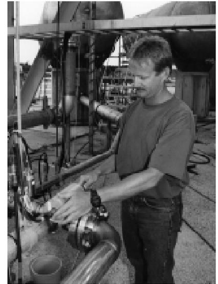
*A KSC employee (above) installs a Universal Signal Conditioning Amplifier (USCA) for testing at the Launch Equipment Test Facility. The USCA is a key component of the Automated Data Acquisition System (ADAS), which includes a circuit board as shown in the photo at left. ADAS monitors temperature, pressure and vibration measurements at the Center's launch pads.*
