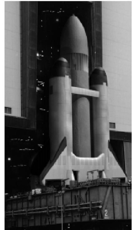
*This is one conceptual view of liquid fly-back boosters, flanking the external tank (center), for the Space Shuttle program.*
