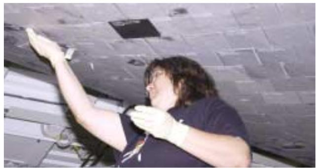
A tile technician inspects tile on orbiter Endeavour in preparation for the next flight.
