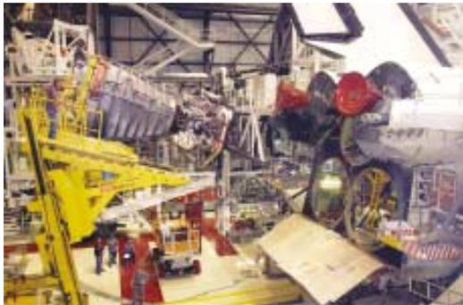
Technicians install the first of three Space Shuttle Main Engines on Atlantis in preparation for mission STS-112.
