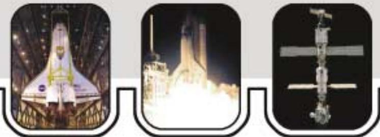
From left: Discovery was suspended by an overhead crane in the VAB prior to stacking with the external tank and solid rocket boosters for Mission STS-92, the Shuttle program's 100th flight; Mission STS-92 launched on Oct. 11, 2000 and delivered the Z-1 Truss to the ISS; a view of the ISS from Endeavour during Mission STS-97 showed the Unity module, newly-installed P6 Integrated Truss Structure and Solar Array Wing-3, that provided power to the Station.
