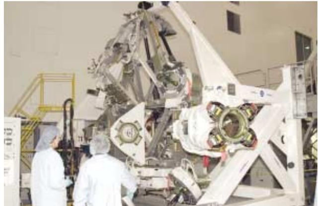
Workers in the Space Station Processing Facility look over the Mobile Base System (MBS), part of the payload on mission STS-111 to the International Space Station.
