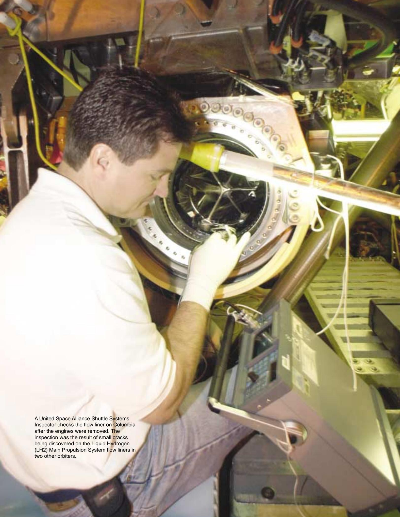
A United Space Alliance Shuttle Systems Inspector checks the flow liner on Columbia after the engines were removed. The inspection was the result of small cracks being discovered on the Liquid Hydrogen (LH2) Main Propulsion System flow liners in two other orbiters.
