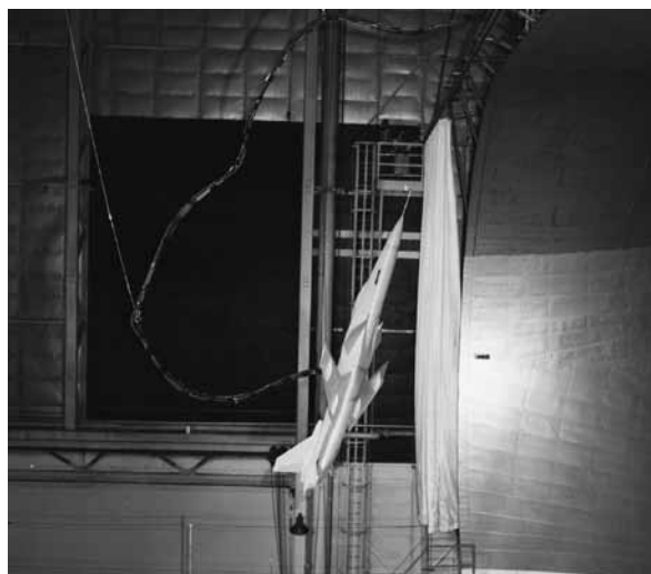
As interest in thrust vectoring intensified in the 1980s, other Langley organizations designed supersonic advanced configurations using thrust vectoring as the primary control concept. This tailless design of a supersonic fighter using pitch- and yaw-vectoring vanes for control was flown at extreme angles of attack during free-flight tests in the Full-Scale Tunnel.
