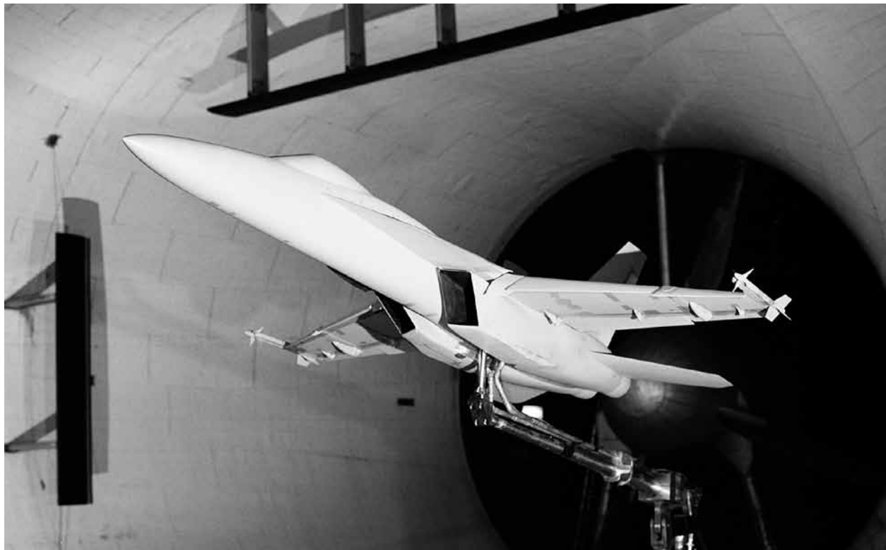
With the transfer of the Langley Full-Scale Tunnel in 1995 to Old Dominion University, NASA's last high-angle-of-attack test program in the facility was a series of force tests for a free-flight model of the F/A-18E.
