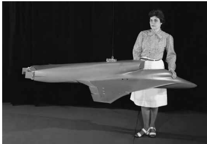
As interest in thrust vectoring intensified in the 1980s, other Langley organizations designed supersonic advanced configurations using thrust vectoring as the primary control concept. This tailless design of a supersonic fighter using pitch- and yaw-vectoring vanes for control was flown at extreme angles of attack during free-flight tests in the Full-Scale Tunnel.
