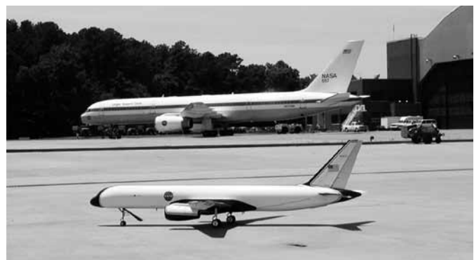
The NASA AirSTAR program is developing a powered free-flight model technique to study upset recovery and other safety issues for commercial transport configurations. Flight tests of generic powered transport models are underway to minimize risk during studies of a scaled model of the test subject.
