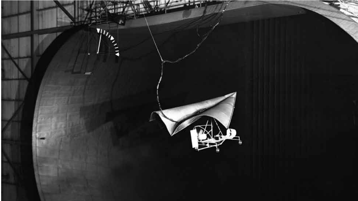
Free-flight model of parawing utility vehicle during tests in the Langley Full-Scale Tunnel. Control was accomplished by tilting the parawing relative to the pilot's platform. After large adverse control effects were discovered using the technique, researchers conceived new roll control concepts using hinged keel members.
