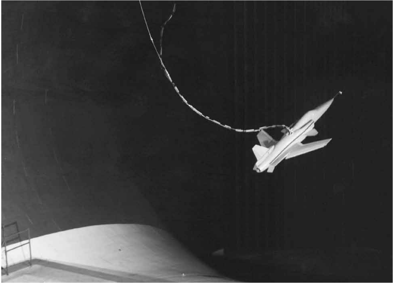
Dynamic free-flight model tests of the X-29 advanced technology demonstrator were conducted in the NASA Langley Full-Scale Tunnel to determine the configuration's dynamic stability and control characteristics. The photograph shows the model flying at a high angle of attack while researchers assess its behavior. Note the large nose-down deflection of the canard surface, an indication of the inherent static instability of the configuration. Active controls using data from an angle-of-attack sensor on the nose boom provided artificial stability.
