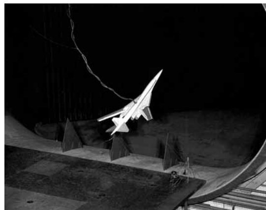
Free-flight model of the Boeing variable-sweep model 733 Supersonic Transport undergoes assessments of dynamic stability and control in the Full-Scale Tunnel. After these tests, Boeing changed its configuration for the SST to a fixed wing design.
