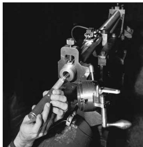
Model, sabot, and cartridge assembly prepared for firing in the Ames Supersonic Free-Flight Tunnel.
