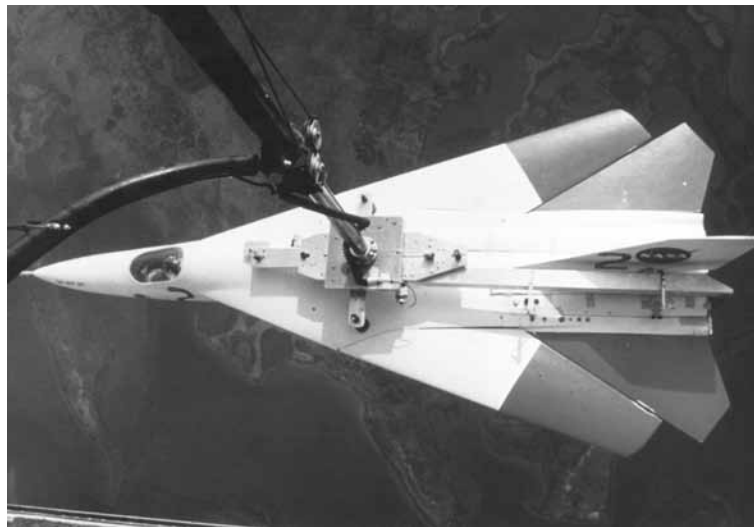
A one-ninth-scale model of the F-111 awaits launch from the helicopter over the Plum Tree Island test site in 1968. Two models were used in the program, which included follow-on NASA research on automatic spin prevention systems after direct support of the F-111 development efforts were completed.
