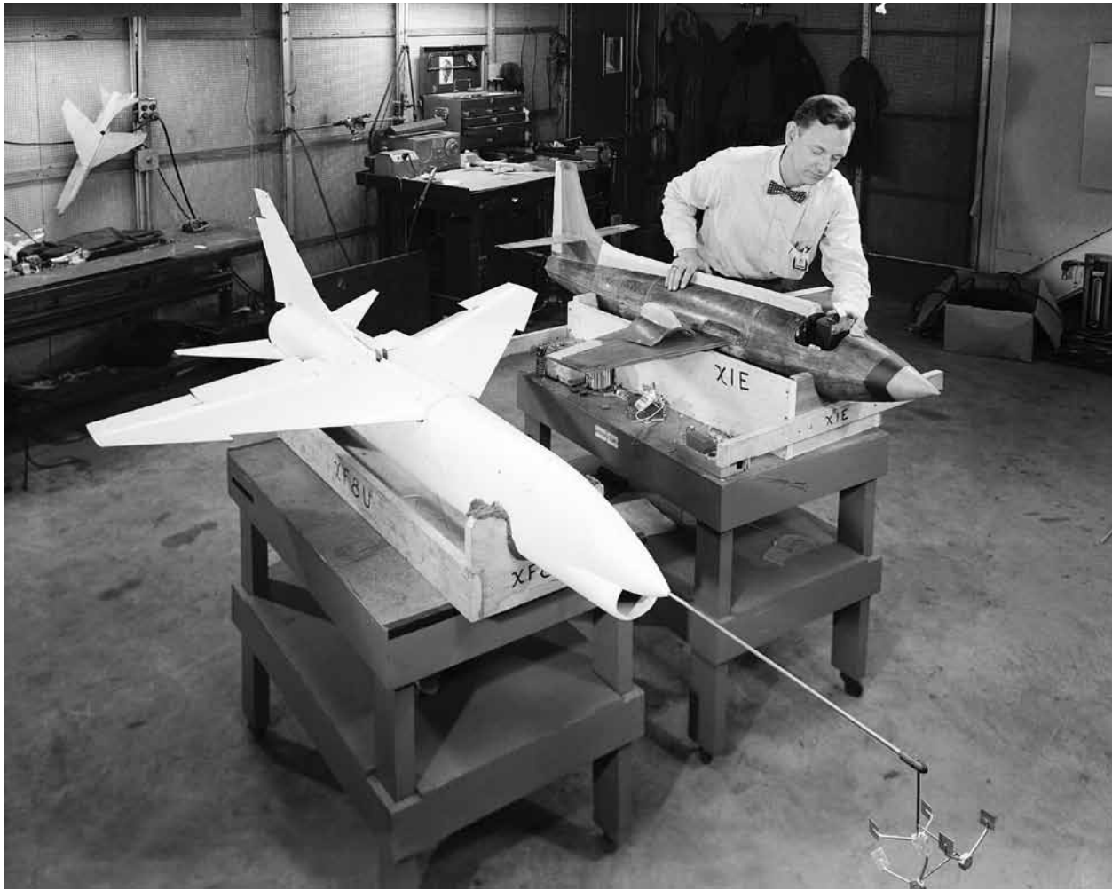
Radio-controlled drop models of the XF8U-1 and the X-1E being prepared for studies of incipient spin behavior using the helicopter drop-model technique in 1958. Note the large flow direction vanes used on the nose boom of the XF8U-1 model. Instrumentation for the drop models was rapidly advanced and miniaturized in subsequent models.
