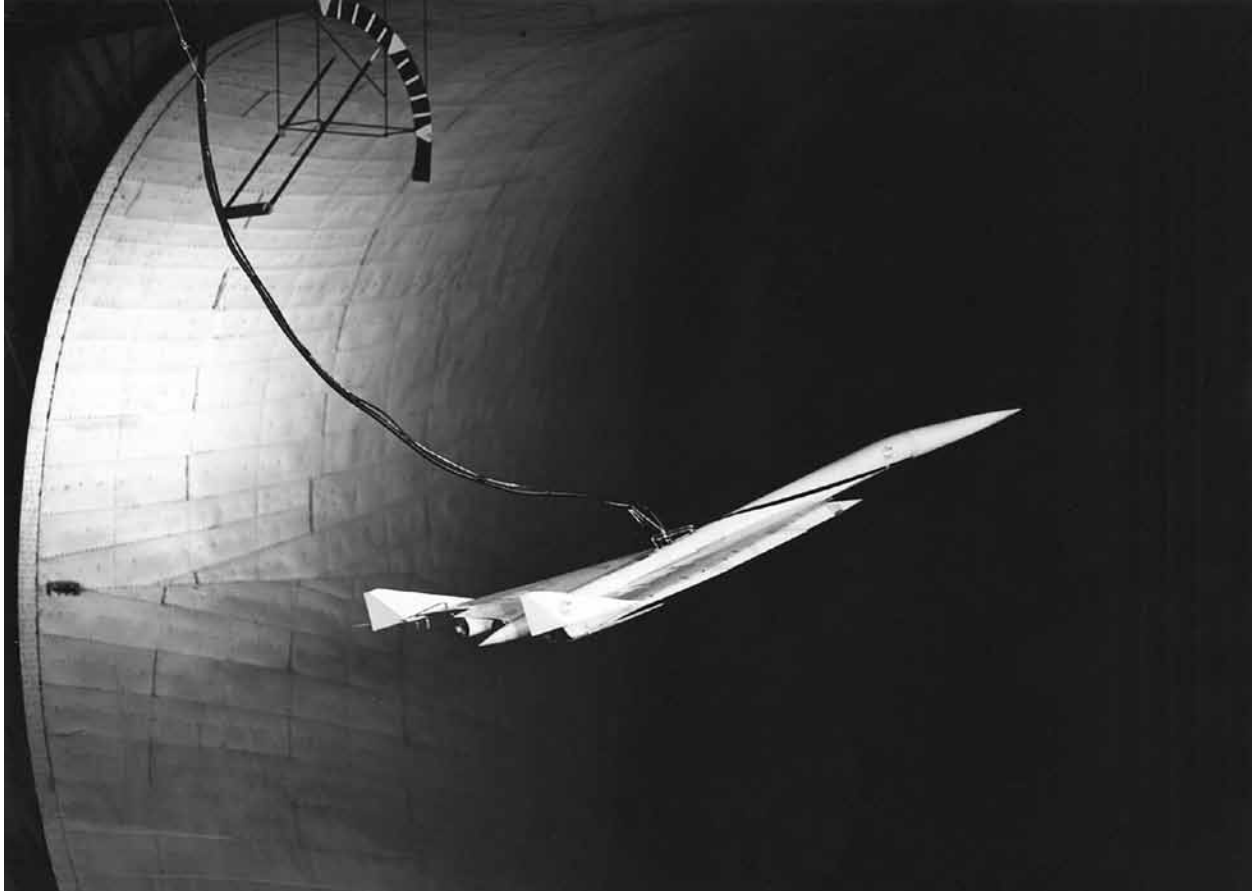
Free-flight model of the NASA Langley SCAT 15F Supersonic Transport in the Full-Scale Tunnel. The SCAT-15 design still represents the most efficient Supersonic Transport configuration.
