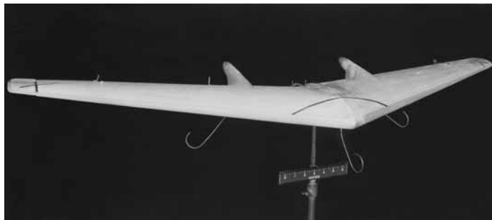
Free-flight model of the Northrop N-9M used in dynamic stability studies in the 12-Foot Free-Flight Tunnel. The test was the first of a series of studies of tailless designs that led to a NACA summary report. Shown here without propellers, the model was also tested for powered conditions.
