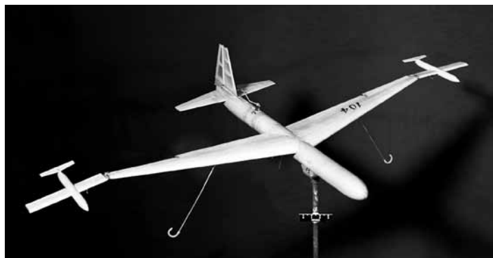
The wingtip-coupling concept was studied in several dynamic stability investigations in the Free-Flight Tunnel. Critical parameters for stability and control such as the fore-and-aft location of the parasite fighters on the bomber's wing tips were identified.
