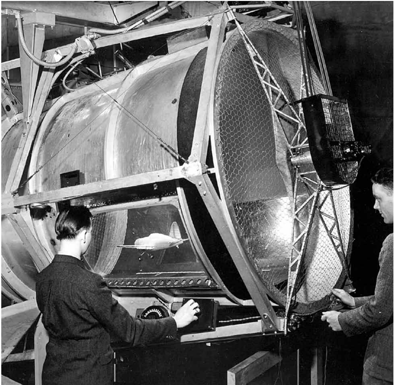
Free-flight tests of a model of the Brewster Buffalo airplane in the 5-Foot Free-Flight Tunnel. The researcher on the left controls the tilt angle and airspeed of the yoke-mounted tunnel, while the evaluation pilot on the right provides control inputs via light flexible cables from his control box to the model.
