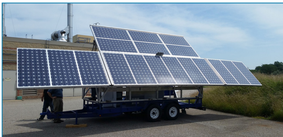
Above: The mobile solar power plant mounted on a trailer. When solar array panels are deployed, they span 512 feet.
