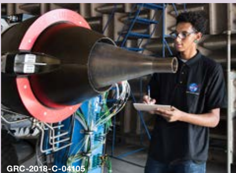
Severino researches test engine noise reduction.
