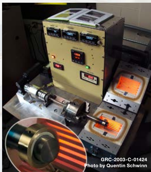
The coating process for PS400.
