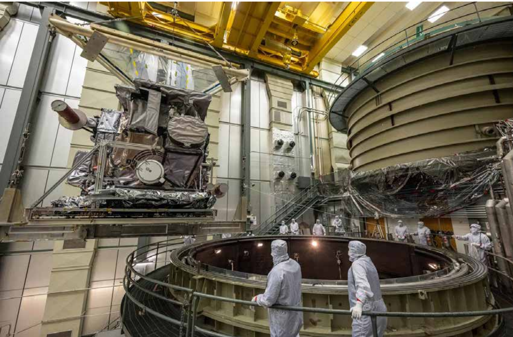
The Geostationary Operational Environmental Satellites (GOES)-T lifted to the 29' x 65' thermal vacuum chamber on September 29, 2020. Photo Credit: Lockheed Martin
