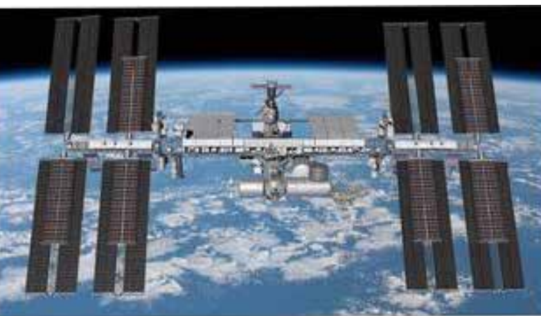
This image shows the planned configuration of six iROSA solar arrays intended to augment power on the International Space Station. The roll-up arrays arrive on the SpaceX-22 resupply mission. Image Credit: NASA/Johnson Space Center/Boeing
