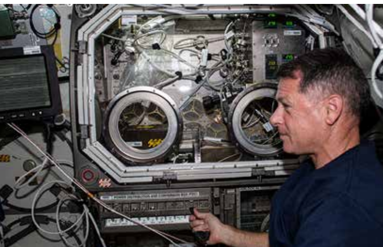
NASA astronaut Shane Kimbrough sets up hardware for the SUBSA physics investigation that examines the mechanisms behind solidification of brazing alloys in microgravity inside the Microgravity Science Glovebox. Photo Credit: NASA
