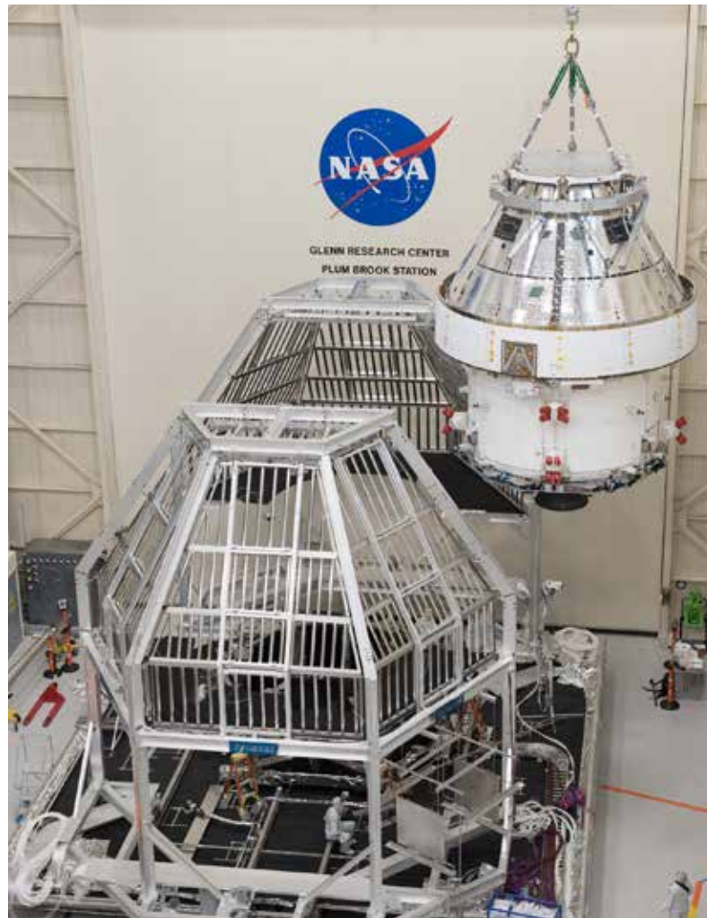
NASA’s Orion spacecraft, the crew module and European-built service module, is lifted into a thermal cage and readied for its move into the vacuum chamber at NASA’s Plum Brook Station for testing. Testing began with a 60-day thermal test, where the spacecraft was subjected to temperatures ranging from -250 to 300-degrees Fahrenheit to ensure it can withstand the harsh environment of space during Artemis missions. Photo Credit: NASA/Marvin Smith
