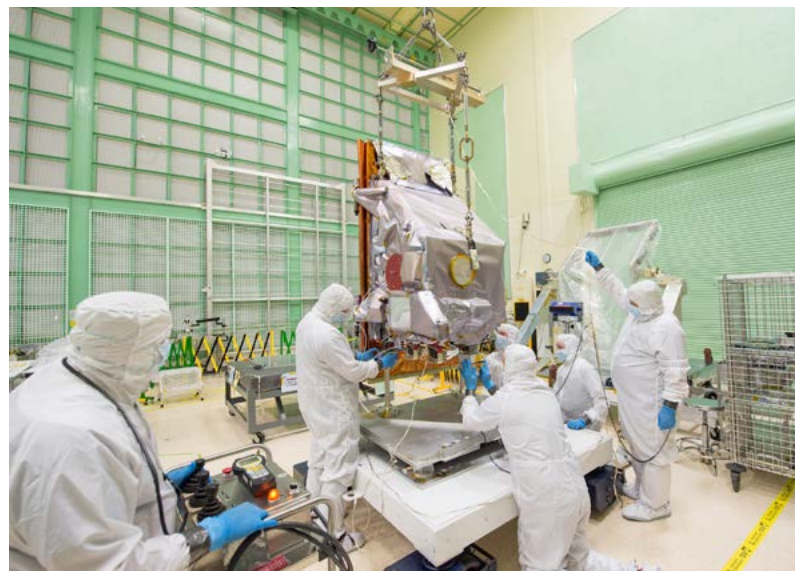
Engineers at the Goddard Space Flight Center prepare the TIRS-2 instrument for integration with Landsat 9 in August 2019. TIRS-2 will measure surface temperatures on Earth from the Landsat 9 satellite. Photo credit: NASA
