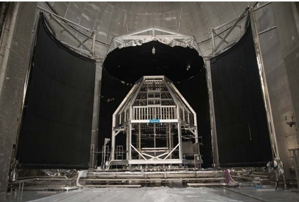
The Space Environments Complex thermal vacuum chamber, located at NASA’s Plum Brook Station in Ohio, stands ready to test the recently completed Orion spacecraft in September 2019. This was Orion’s last major testing before being integrated with the Space Launch System for Artemis 1. The vacuum chamber—the largest in the world—will replicate the extreme hot and cold temperatures that Orion will experience while flying through space. Photo credit: NASA
