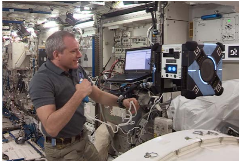
On June 14, 2019, Bumble (the cube to the right of astronaut David Saint-Jacques, of the Canadian Space Agency, and the laptop) became the first of NASA's Astrobees robots to fly under its own power in space. Astrobees robots, which can move in any direction and rotate on an axis, will help the astronauts test new technologies and perform routine work aboard the ISS. Photo credit: NASA.
