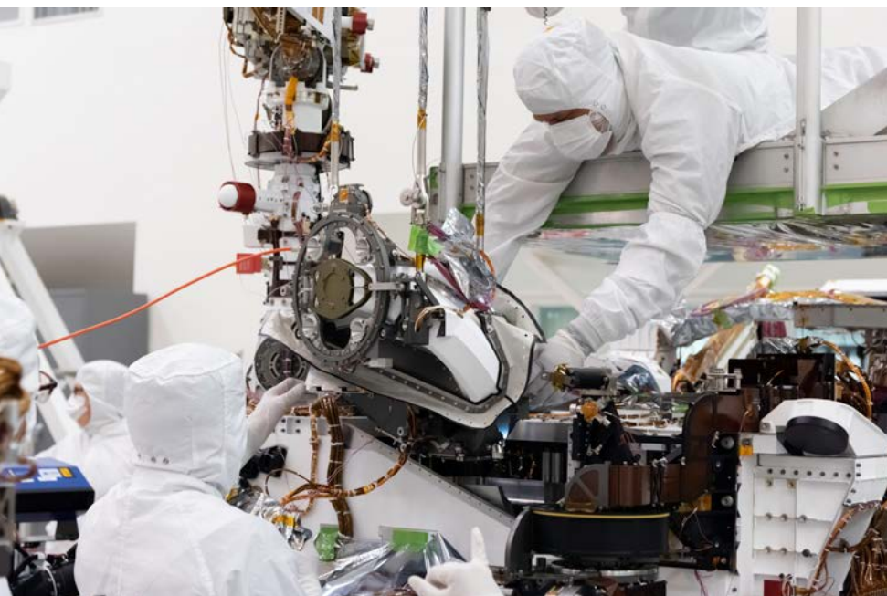
Engineers at the Jet Propulsion Laboratory attach the bit carousel, which lies at the heart of the Mars 2020's Sample Caching System, to the front end of the rover on August 5, 2019. The carousel contains the tools that the coring drill will use to sample the Martian surface and is the gateway through which the samples will enter the rover for assessment and processing. Photo credit: NASA/JPL-Caltech
