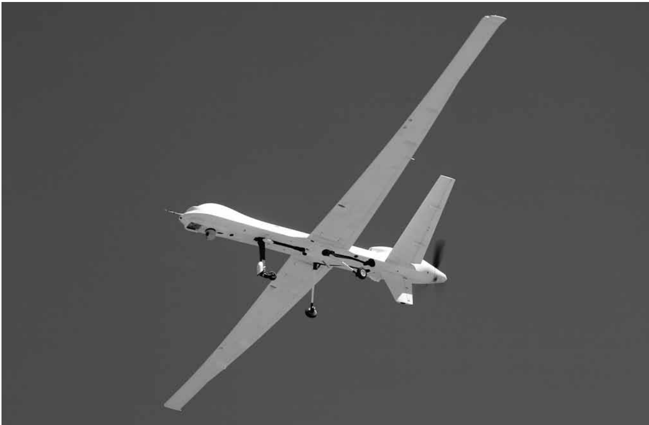
The Altair vehicle was the first UAV to feature triple-redundant avionics as well as a fault-tolerant flight control system. NASA
