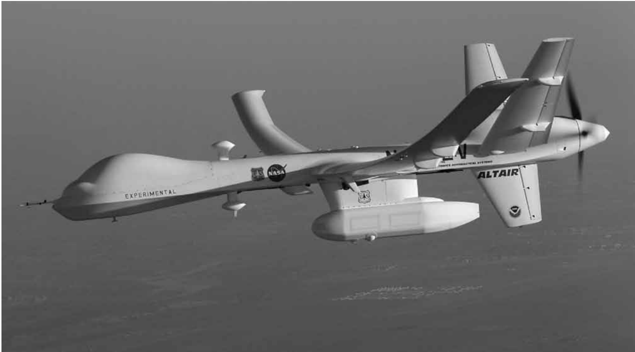
The Altair carried the sensor pod on a ventral centerline pylon. Sensor data is autonomously processed with georectified topographical information to create a fire-intensity map.
