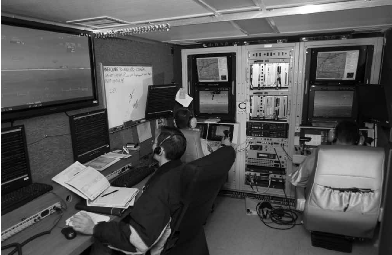
The ground control station includes consoles for two pilots and positions for scientists and engineers. NASA
