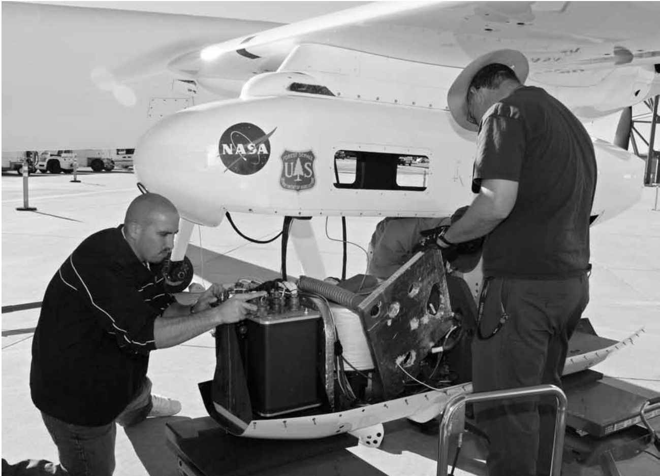
Ikhana ground crewmen Gus Carreno and James Smith load the thermal-infrared imaging scanner pallet into the Ikhana's underwing payload pod.
