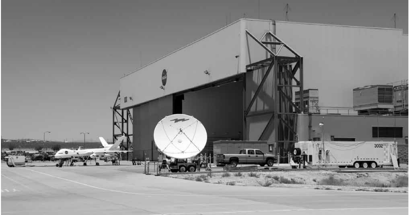
The Ikhana is flown from a ground control station, visible at right. A Ku-band satellite communications system provides data uplink and downlink capability.
