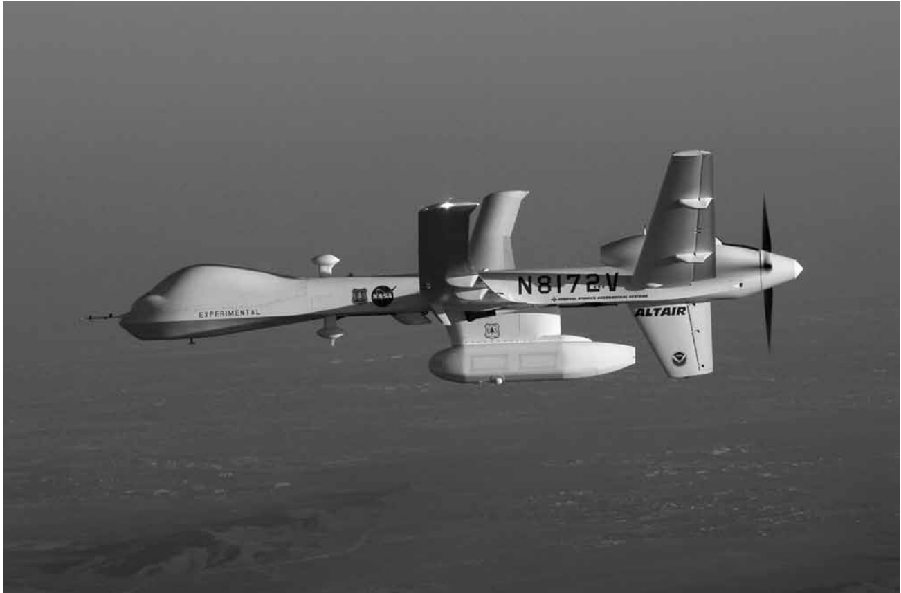
The Altair was flown over a controlled burn near Yosemite National Park as well as a nearby wildfire to confirm satellite-based fire-detection information and to test the AMS sensor.
