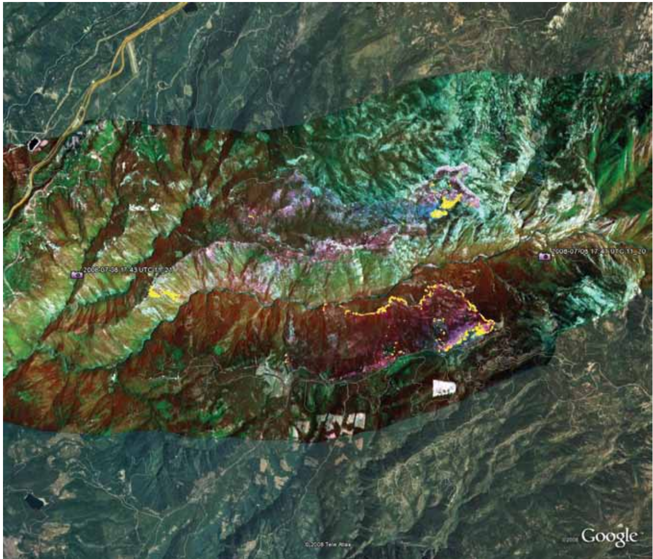
Fires over the American River Fire Complex in Placer County, Calif., are seen as taken by the AMS wildfire scanner aboard the Ikhana, July 8, 2008. The yellow areas depict active fire areas. The image provides officials not only with fire information but also with vegetation-type and burned-area information.
