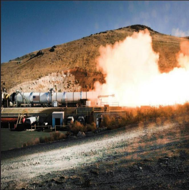
DM-2 Static Motor Firing in Utah
