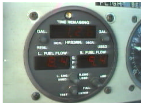
Figure 8.6 Fuel Flow Meters on Test Aircraft
