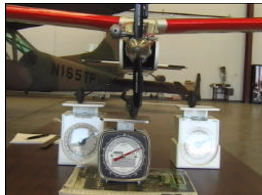
Weighing the Aircraft
