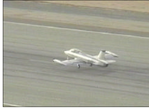
Figure 6.3 Takeoff Distance Determination from Chase Aircraft
