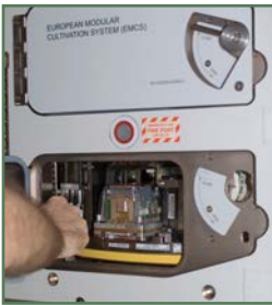
Astronaut Michael E. Lopez-Alegria, Expedition 14 commander and NASA space station science officer, replaces the European Modular Cultivation System (EMCS) Experiment Container (EC) in the Destiny laboratory of the International Space Station.
