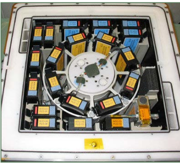
Kubik with centrifuge configuration loaded with experiment containers. Image courtesy of ESA.
