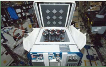
Photograph of CGBA during Increment 33 showing open containment volume and sample canisters. Image courtesy of NASA.
