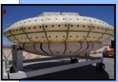
Robotic class supersonic inflatable aerodynamic decelerator prototype after rapid inflation test at China Lake
