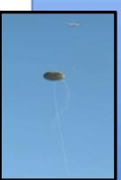
Helicopter, cargo parachute, mass simulator and attach cabling during first Parachute Development Verification test at China Lake
