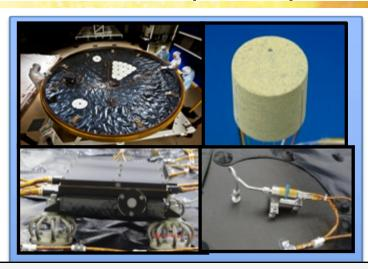
Image group: Top left photo of NASA Team preps for launch of Mars rover and check of sensors. Top right image is of thermal plugs containing instruments to measure changes in thickness and in-depth temperatures. Bottom right photo of pressure transducers attached to the inside of the aeroshell structure. Bottom left image is the custom-built electronics box collects the <1 MB of MEDLI data.
