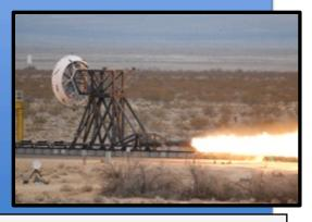
In March 2012, NASA performed a trial run on a rocket sled test fixture, powered by rockets, to replicate the forces a supersonic spacecraft would experience prior to landing.
