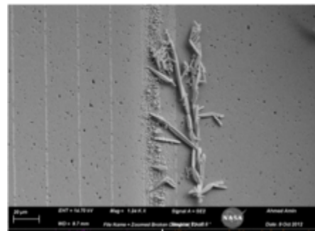
Fig. 5: Tin Dendrite (PME 0.8V WLT, 18 mins)
