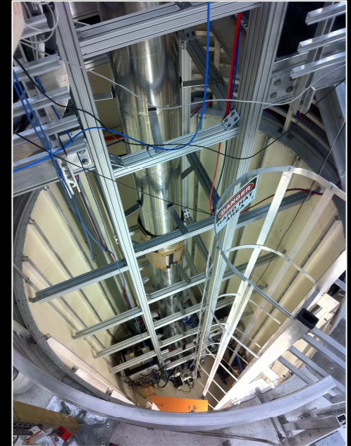
Stanford University drop tower, which is being used to test a Goddard-designed laser system critical in atom-optics technology.
