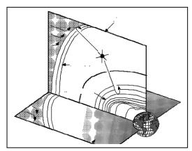
The IMAGE spacecraft (shown as the 'star' in the figure) contains an instrument called the Radio Plasma Imager (RPI). This instrument sends out a powerful pulse of radio energy (the fish hook-shaped lines) at frequencies from 3,000 to 3 million cycles per second (Hertz). When the echos from these pulses are later received by the instrument, they can be analyzed to find the location and density of the plasma that reflected them.
