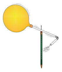
Demonstrate the action-reaction principle by inserting a pin through the straw and into a pencil eraser. Inflate the balloon, and it will pinwheel around the pencil as air rushes out. Compare this to the straight thrust produced by the balloon in the rocket cars.
