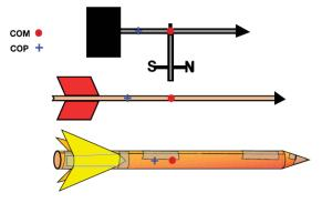
The positions of center of mass (red dot) and center of pressure (blue +) are shown for a weather vane, arrow, and rocket. The center of pressure is to the rear of the center of mass in each device. This enables them to point into the wind.
