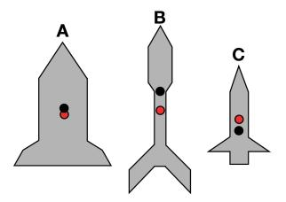
Rocket B is the most stable rocket. Rocket C will definitely tumble in flight. Rocket A will probably fly on a crooked path. Any cross winds encountered by the rocket as it climbs will cause it to go off course.
