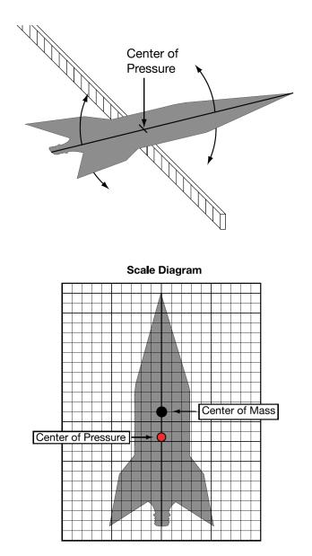
In flight, the rocket will try to tumble around its center of mass. If the center of pressure is properly placed, the rocket will fly straight instead. More air pressure will be exerted on the lower end of the rocket than on the upper end. This keeps the lower end down and the nose pointed up!
