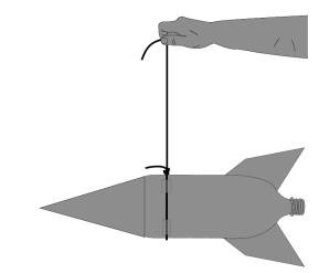
When designing a stable rocket, the center of mass must be to the front and the center of pressure must be to the rear.
