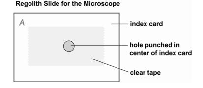
tape, making one slide for each sample. The sample from container "A" should be placed on the index card marked "A", the sample from container "B" should be placed on the index card marked "B", and the same for container "C".
