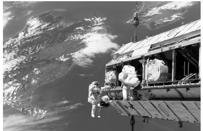
Astronauts work on part of the truss of the International Space Station during STS-115. Notice the triangle-shaped structure inside the truss.
