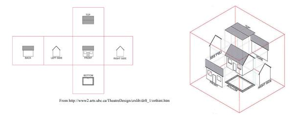
Isometric Drawing is a form of 3-D drawing in which there are three types of lines: vertical lines, 30° lines to the right and 30° lines to the left. Isometric graph paper makes it easy to draw neat, accurate images of design ideas. See the next page for a sample.
