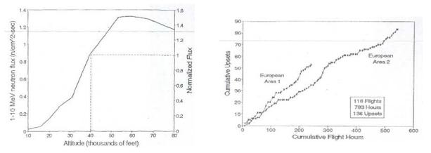
The left-hand curve gives the number of neutrons that pass through each square centimeter of surface every second (the neutron flux). The right-hand plot gives the cumulative number of memory upsets at an altitude of 30,000 feet after a given number of hours in the air.
