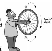
2. Before spinning the wheel, try tilting the wheel left and right, from vertical to horizontal. Also, try twisting it around while keeping it vertical. Notice any resistance from the wheel?
