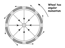
centripetal force combine to give the object angular momentum. Angular momentum is what makes the bike wheel tend to keep spinning in the same plane, that is, going in the same direction, as when force was first applied to get it spinning. In our Trick 3, that plane was more or less vertical, so that is the orientation the bike wheel wants to keep, in apparent defiance of gravity!
