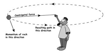
Now, put these ideas together and spin the bike wheel. The rim and tire of the wheel are like a bunch of rocks fused together into a circle and tied to the center (hub) by spokes instead of string. Each part of the outside of the wheel has momentum and wants to keep going in the direction it was pushed. But it can't, because it is being pulled in toward the center by the spokes exerting centripetal force.
