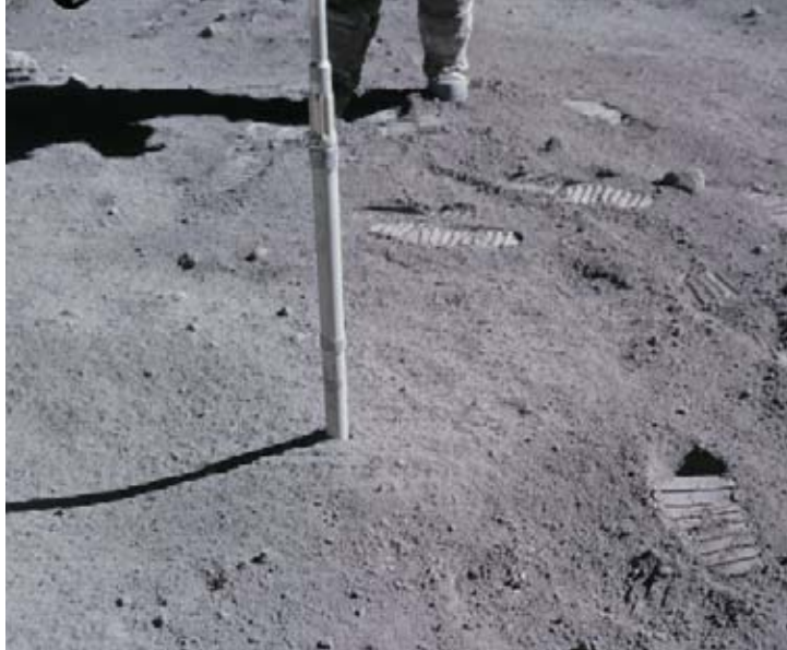
Apollo 16 astronaut Charlie Duke (feet shown) drives a core sample tube into the lunar regolith.
