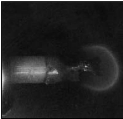
The familiar shape of a candle flame on Earth is caused by buoyancy-driven convection. In microgravity, a candle flame assumes a spherical shape as fresh oxidizer reaches it by diffusion processes.
