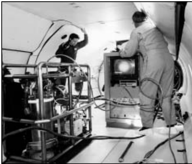
Researchers observe the float package and data rack of a superfluid helium experiment on a parabolic aircraft flight.
