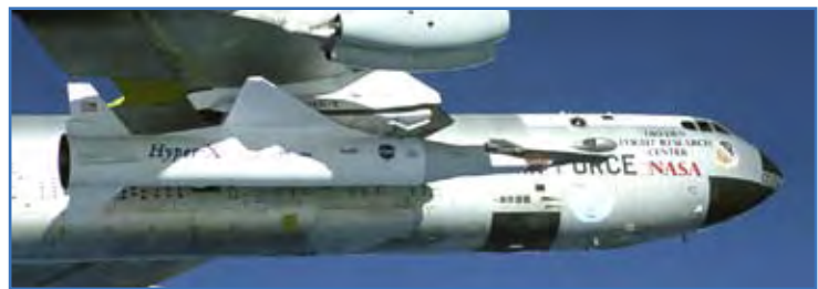
A B-52 carried the X-43 , riding on the tip of a Pegasus rocket, to 40,000 feet where the Pegasus was launched. At 95,000 feet, the X-43 was released from the rocket and flew under its own power to reach an altitude of 110,000 feet at almost Mach 9.6, or nearly 7,000 miles (11,265 kilometers) per hour.
