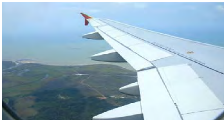
Flaps on a plane help to create drag.
