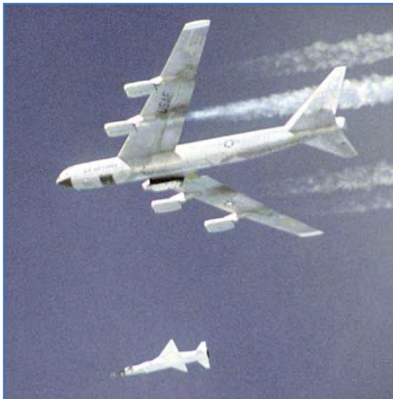
The X-43 was launched from a B-52 and flew at 7,000 mph (11,265 kilometers per hour) under its own power.
