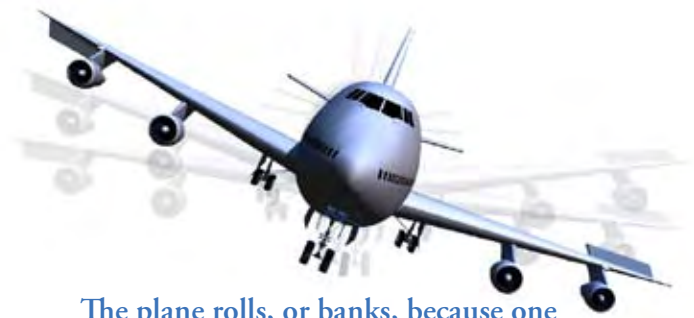
The plane rolls, or banks, because one aileron is up and one aileron is down.
