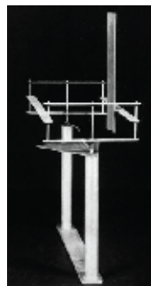
The drag balance tested the airfoil for drag.
