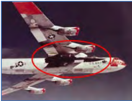
The B-52 carried the X-15 under its wing until it reached a high altitude. Then, the X-15 was dropped, and its rocket engines took over.
