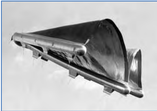
Photo of Rogallo's flexible wing (Parawing), which was tested by NASA.
