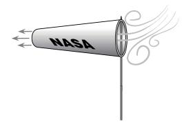
A wind sock is a type of kite used to detect wind direction. It is a tapered tube of cloth that is held open at one end by a stiff ring. Wind is directed down the tube, causing the narrow end to point in the same direction the wind is blowing. Brightly colored wind socks are used at airports to help pilots determine the wind direction along the ground. *Meteorologists* use wind direction to help predict the weather.
