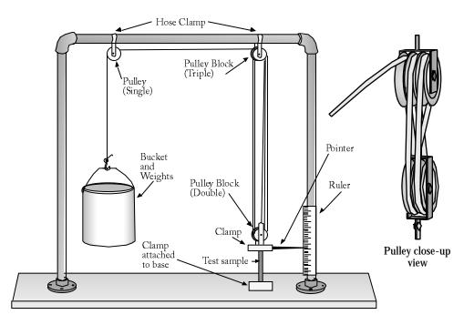
the bucket. The mechanical advantage of the pulley arrangement magnifies the actual pull (tensile force) on the sample five times. Record the tensile force (the weight in the bucket multiplied by five) and the position of the pointer. The position of the pointer indicates how much the fabric stretches as the force increases. Add more weight and record the data. Continue this process until the sample breaks or you run out of weights. Create a graph to demonstrate the performance of the material.
