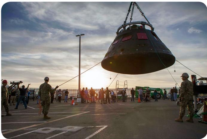
The Orion crew module is moved by crane Dec. 13 from its crew module recovery cradle and placed in the crew module transportation fixture at the Mole Pier at Naval Base San Diego in California. (NASA)
