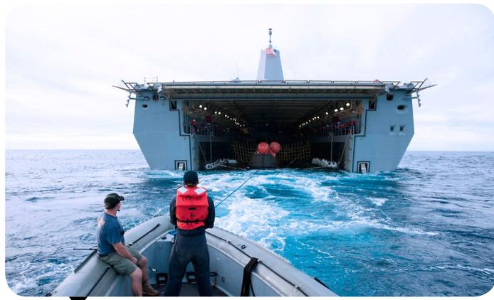
Recovery team members in a Zodiac boat help guide NASA's Orion spacecraft into the well deck of the USS Anchorage following its splashdown in the Pacific Ocean. (U.S. Navy)
