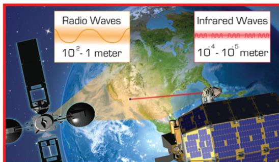
This reduction in antenna size applies for both ground and space receivers, which reduces satellite size and mass. Laser communication terminals can support higher data rates with lower mass, volume and power requirements, a cost savings for future missions. For laser communications to become standard, NASA first must prove the concept is a viable option. NASA's LLCD mission will test this concept.
