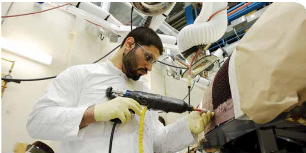
Textron technicians apply the Avcoat™ material by "gunning" the material into each of the 320,000 individual cells of the honeycomb structure.
