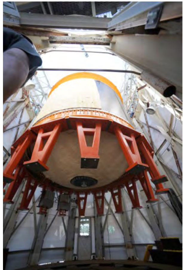
The 18-foot-diameter (5.5-meter) cylinder-shaped composite cryotank being lowered into a structural test stand at the Marshall Center.
