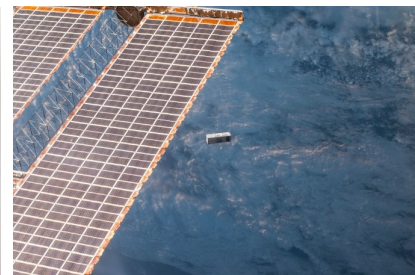
TechEdSat-3p deploys from the Japanese Small Satellite Orbital Deployer aboard the International Space Station.
