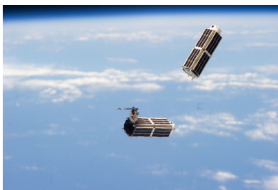
Two of the 28 Planet Labs Dove satellites that make up the Flock 1 constellation are seen launching into orbit earlier this year from the space station.
