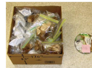
Example of volume reduction /stable tile for mixed trash (Gen 1 HMC tile)
