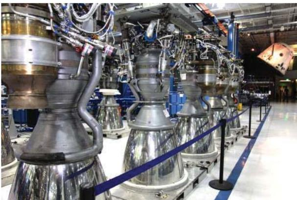
Falcon 9 is the only vehicle currently flying with engine out capability. The nine-engine architecture on the first stage is an improved version of the design employed by the Saturn I and Saturn V rockets of the Apollo program, which had flawless flight records in spite of engine losses.
