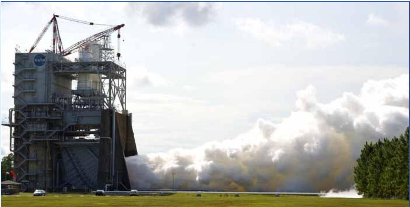
J-2X Engine No. 10002 is test fired for the final time on the A-1 Test Stand at NASA's Stennis Space Center. The 330-second test was the last in a series of gimbal, or pivot, tests on the engine. Following the removal of this engine, the test stand will be modified to begin RS-25 engine testing. J-2X testing has provided valuable data and experience for the team developing the RS-25 engine, which will power the core stage of NASA's new Space Launch System.
