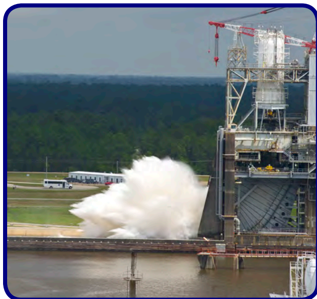
Image Caption: J-2X Engine No. 10002 was test fired on April 17, 2013, at Stennis Space Center. The J-2X is designed to power the second stage of the 130-metric ton heavy-lift version of the Space Launch System (SLS). J-2X testing provided valuable data and experience for the team developing the RS-25 engine, which will power the core stage of NASA's new SLS. (Credit: NASA)
