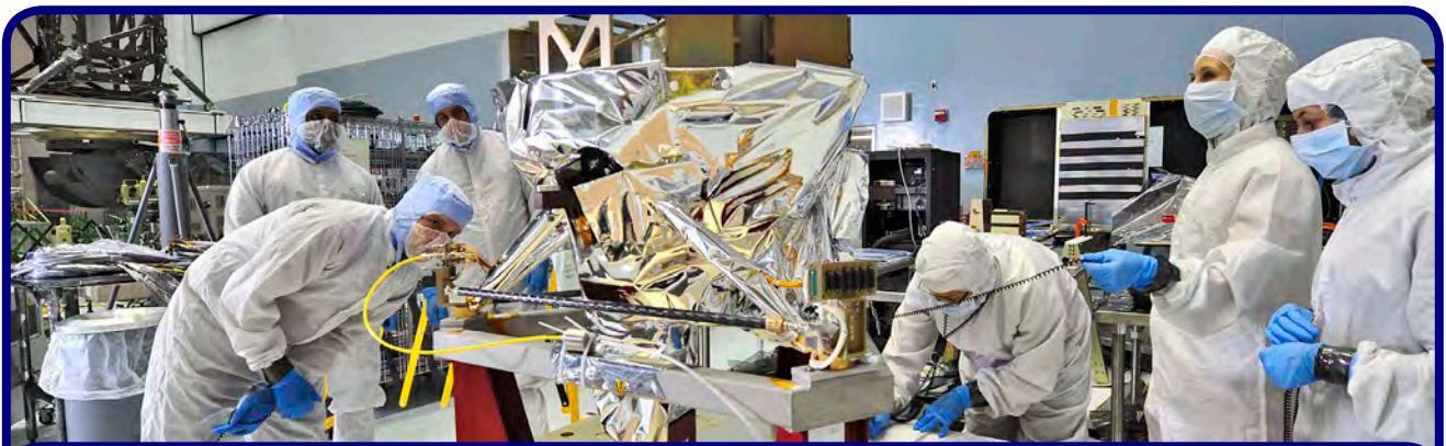
Image Caption: Contamination control engineers conduct a review of the James Webb Space Telescope's Mid-Infrared Instrument, as part of the standard receiving inspection. They are looking for the tiniest traces of dust or contamination which would have to be remedied because cleanliness is critical for such a sensitive instrument. (Credit: NASA/Chris Gunn)
