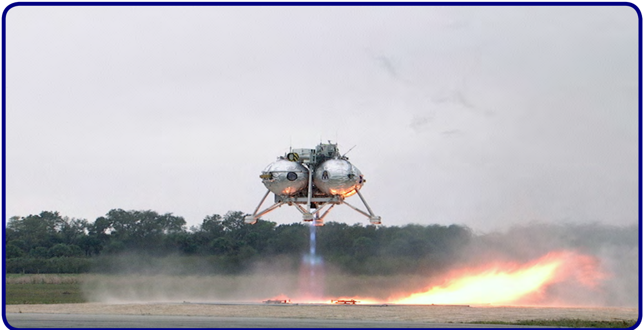
Image Caption: The Morpheus lander ignites its methane and oxygen-powered engine and lifts off to begin a free flight test at NASA's KSC in Florida. The Johnson Space Center-based project is testing new technologies in propulsion and guidance systems in the unique testbed. (Credit: NASA/Frankie Martin)
