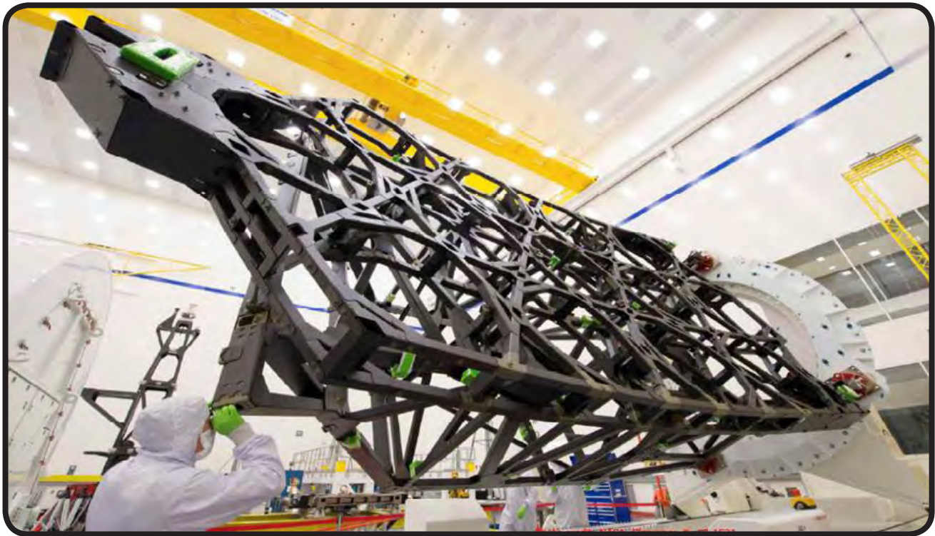
Image Caption: The JWST flight backplane center section and backplane support fixture on a rollover fixture at Northrop Grumman. The hardware pictured here has passed its acceptance testing and is being readied for attaching the primary mirror wings and secondary mirror support struts. (Credit: Northrop Grumman Aerospace Systems)
