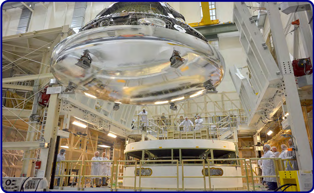
Image Caption: The Orion crew module for EFT-1 shown in the Final Assembly and System Testing (FAST) Cell, positioned over the service module just prior to mating the two sections together. The FAST cell is where the integrated crew and service modules are put through their final system tests. (Credit: NASA/Rad Sinyak)
