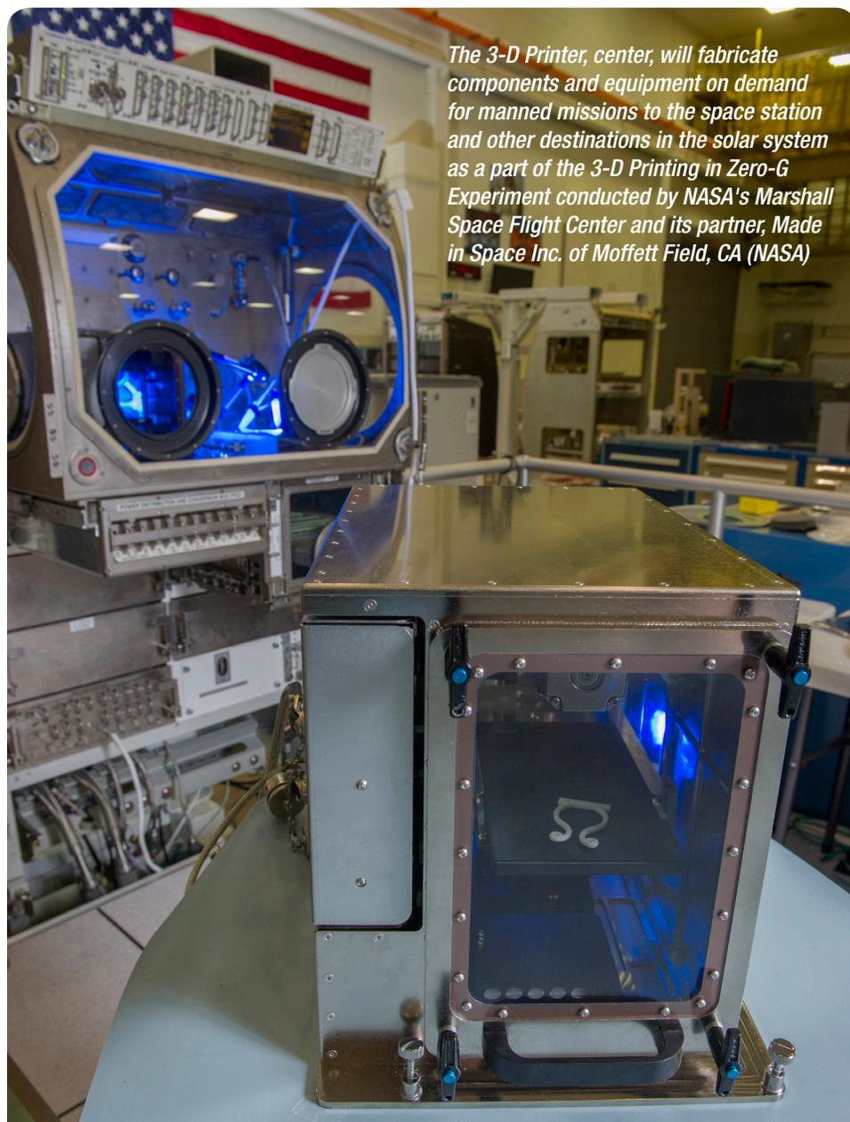
*The 3-D Printer, center, will fabricate components and equipment on demand for manned missions to the space station and other destinations in the solar system as a part of the 3-D Printing in Zero-G Experiment conducted by NASA's Marshall Space Flight Center and its partner, Made in Space Inc. of Moffett Field, CA (NASA)*
