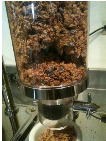
Figure 5: A demonstration of the granular physics phenomenon of "jamming" in a cereal dispenser.
