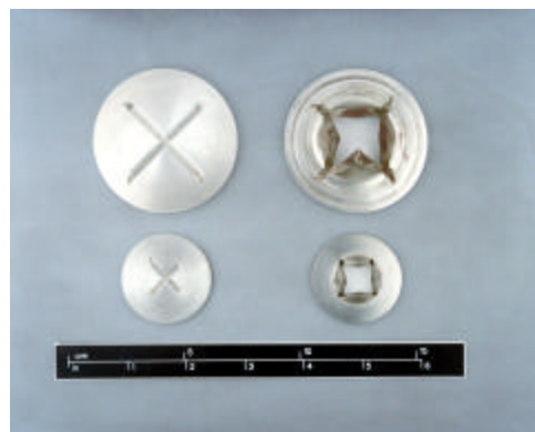
Shown above are .50-cal and 1-in. sabots in both assembled and separated modes. These highly engineered, precision-machined plastic parts are designed to protect the projectile from barrel friction/abrasion, and provide an effective gas seal up to the exit point into the expansion tank.
