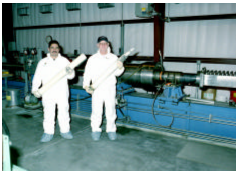
HVI team members display two high-density polyethylene pistons, one before and one after firing. Behind them is the 1-in .LGG.
