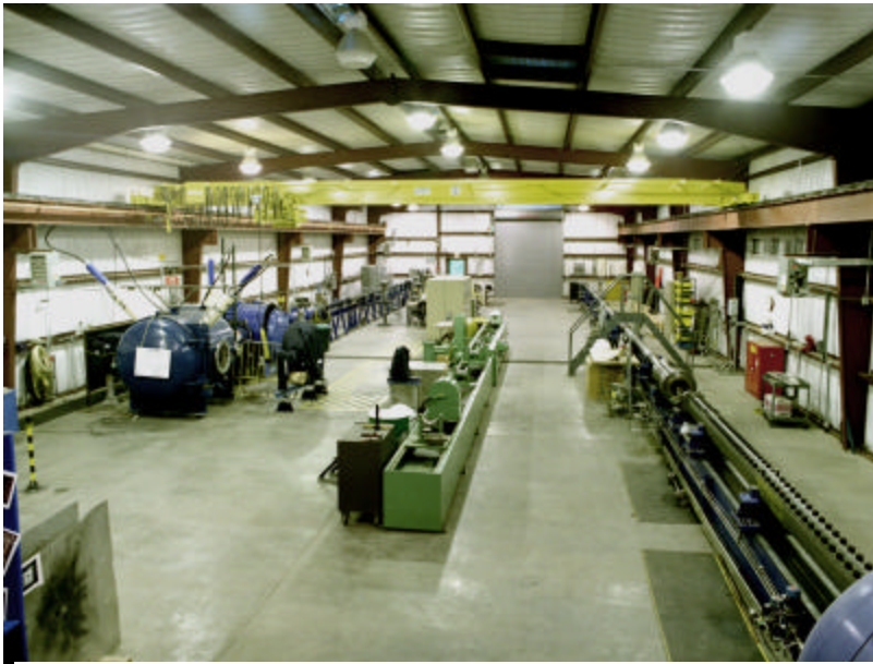
Inside the HVI facility, looking from the muzzle ends of the .50 cal. (left) and 1-in. cal. (right) guns. The precision barrel honer is in the middle.
