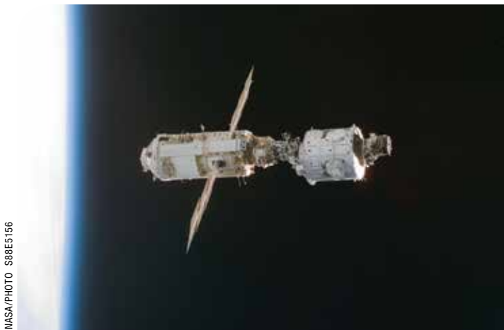
The mated Russian-built Zarya (left) and U.S.-built Unity modules are backdropped against the blackness of space over Earth's horizon shortly after leaving Endeavour 's cargo bay.
