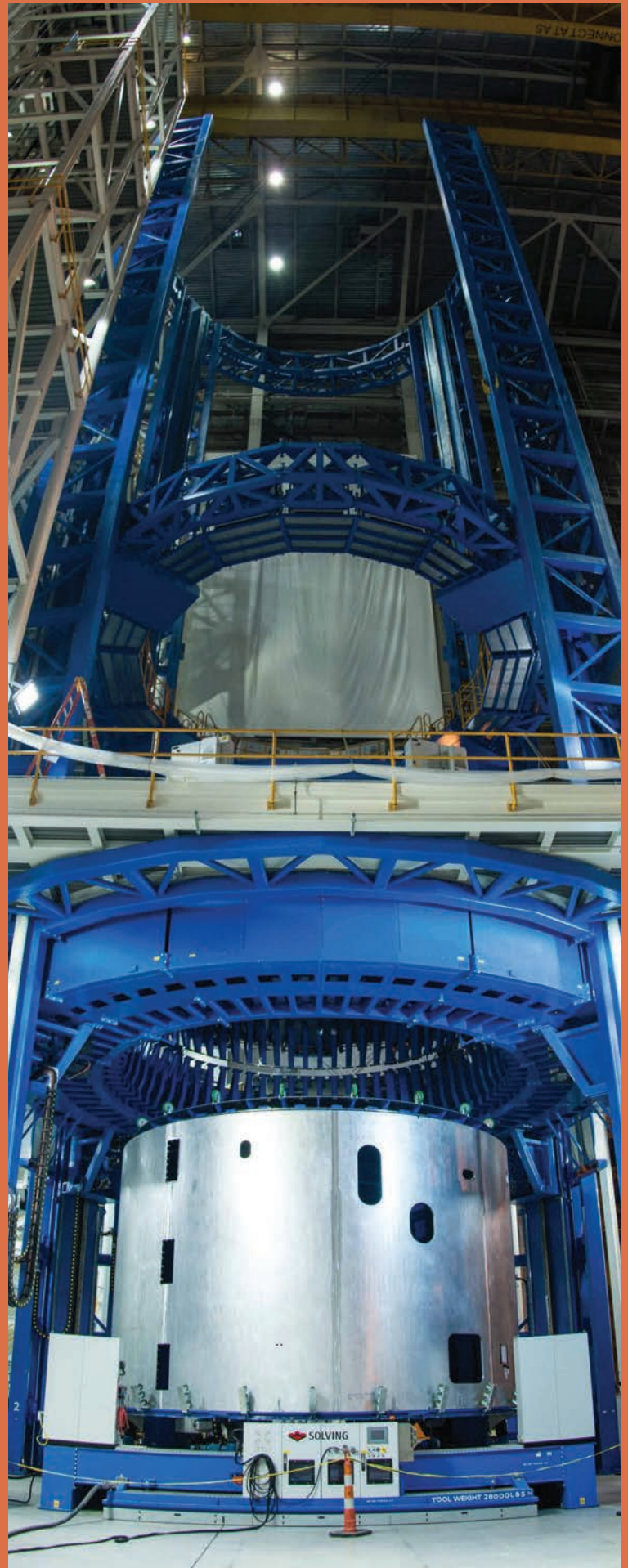
While on a tour of Michoud, guests get a chance to see the engine section weld confidence article in the world's largest welding tool, the Vertical Assembly Center.
