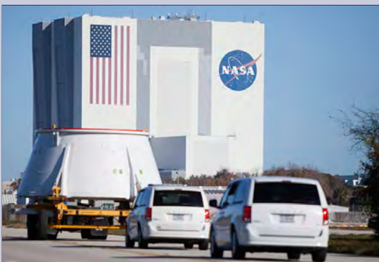
An aft skirt similar to one that will be used on a solid rocket booster (SRB) for NASA's Space Launch System rocket, was transported by NASA and Jacobs engineers and technicians on the Test and Operations Support Contract on Jan. 20, to the Rotation, Processing and Surge Facility (RPSF) at NASA's Kennedy Space Center in Florida. At the RPSF, the aft skirt will be inspected and undergo limited processing to prepare for SRB pathfinder operations. The pathfinder operations will help to test recent upgrades to the RPSF facility as the center prepares for Exploration Mission-1, deep-space missions, and the journey to Mars. Photo credit: NASA/Bill White
