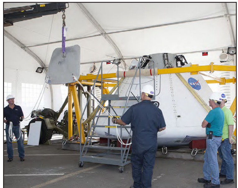
Workers prepared for a simulated fit check of the hatch cover on the Orion boilerplate test vehicle May 13, 2014, inside a protective structure at the Mole Pier at the Naval Base San Diego in California.
