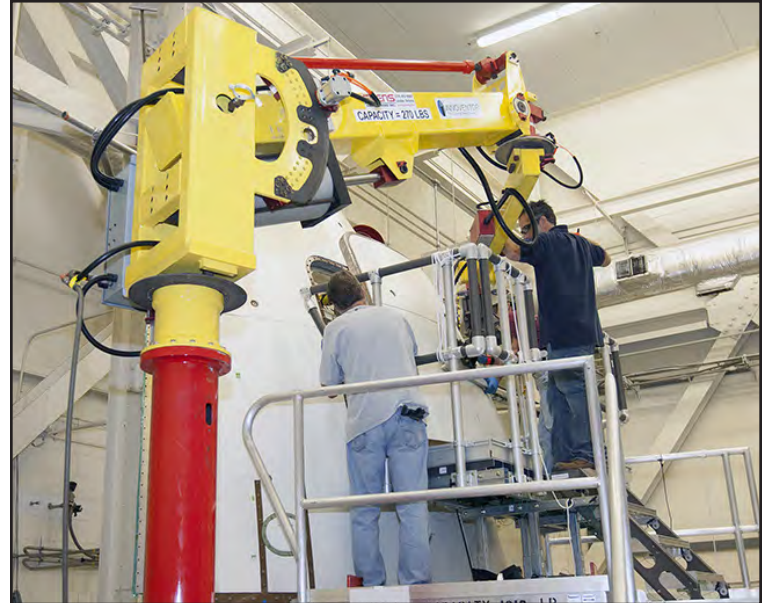
Inside the Vehicle Assembly Building at Kennedy Space Center, engineers and technicians performed a GIZMO demonstration test May 1 on the ground test article Launch Abort System, ogive panel and an Orion crew module simulator to confirm that the GIZMO can meet the reach and handling requirements for the task.
