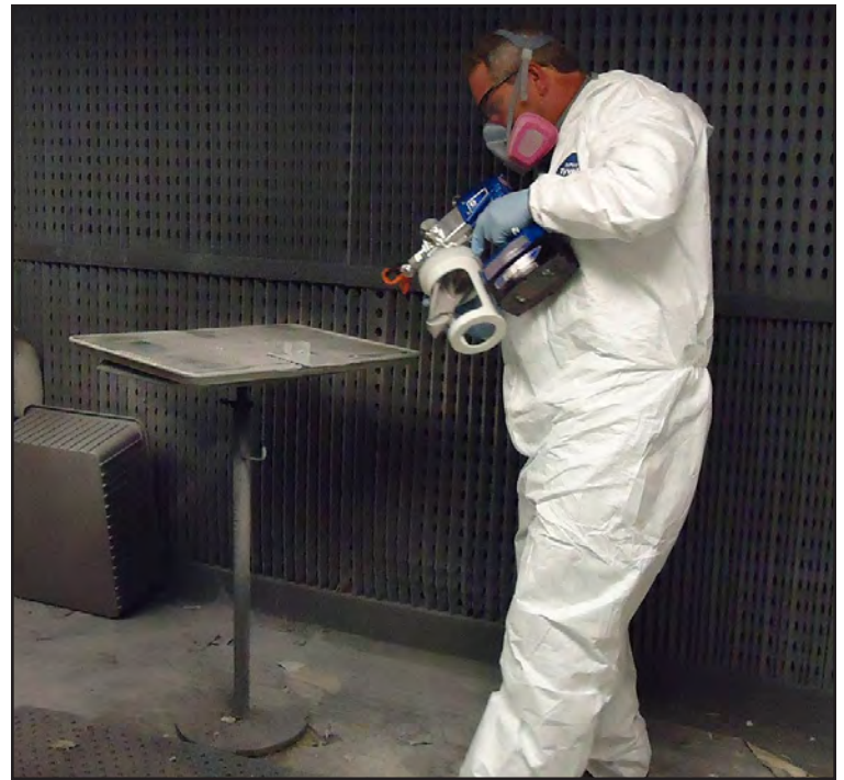
A protective coating is sprayed on a sample panel for testing at the Beachside Atmospheric Test Facility.
