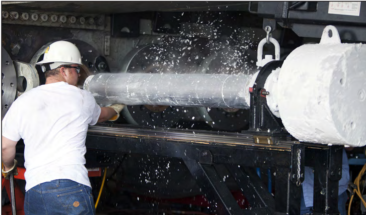
On April 17, ground support technicians used a special work stand to guide an ice-covered roller bearing shaft for insertion on the crawler-transporter 2 inside the Vehicle Assembly Building at Kennedy Space Center.
