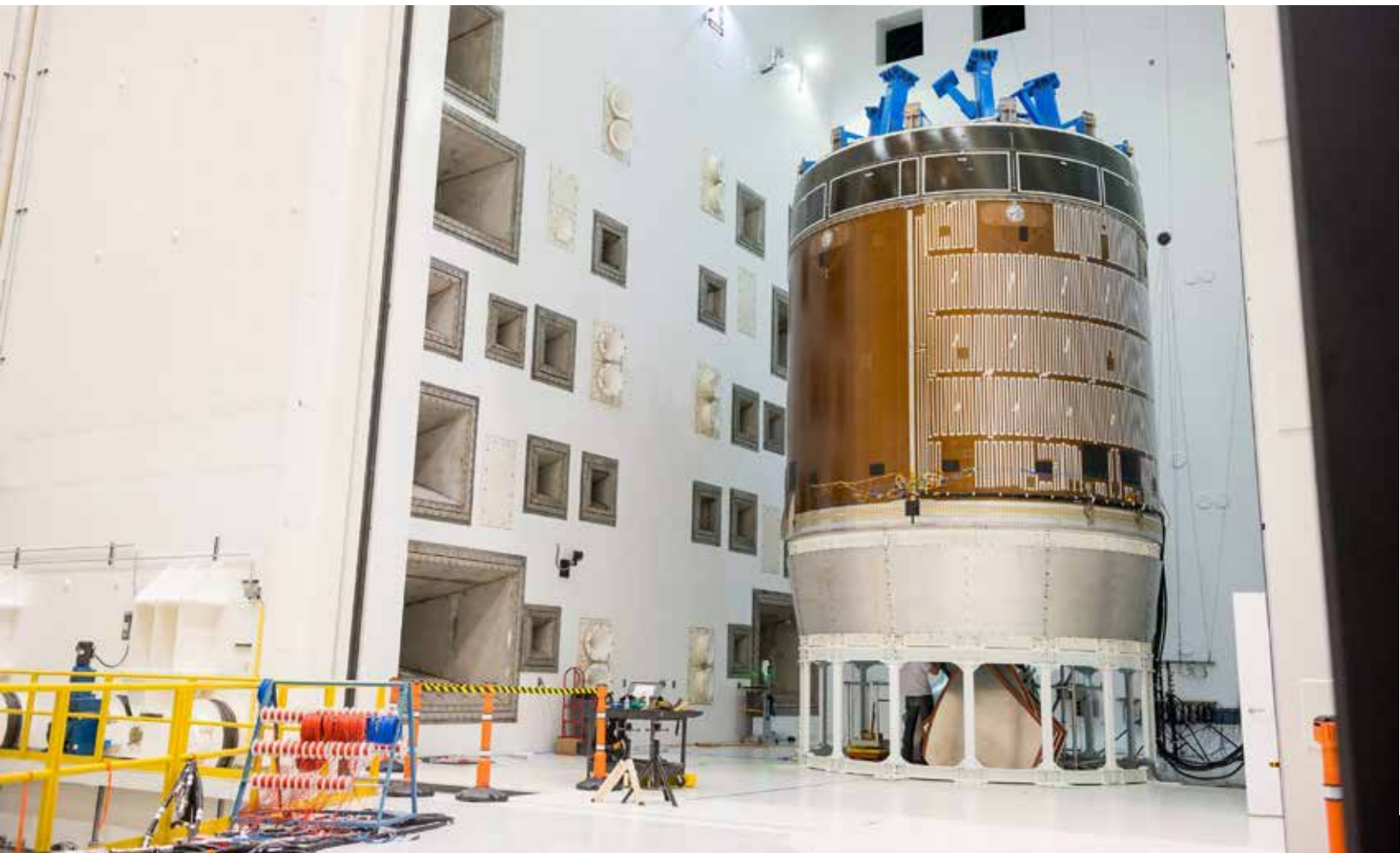
Pictured above: The service module test article sits in the RATF at Glenn's Plum Brook Station ahead of testing. The blue structure sitting on top of the test article is a mass simulator that represents the Orion crew module.
